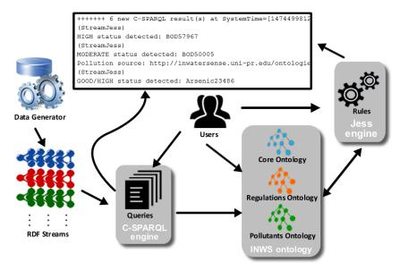
Fig. 1. StreamJess architecture
